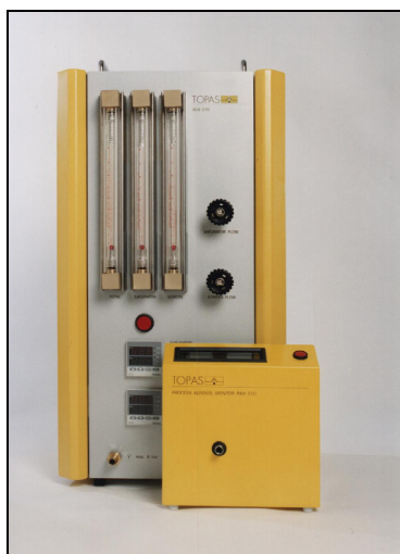
Online Monitoring of Particle Size and Concentration the Monodisperse Aerosol with the Process Aerosol Monitor PAM 510 Directly Connected to the Outlet of a SLG 270
