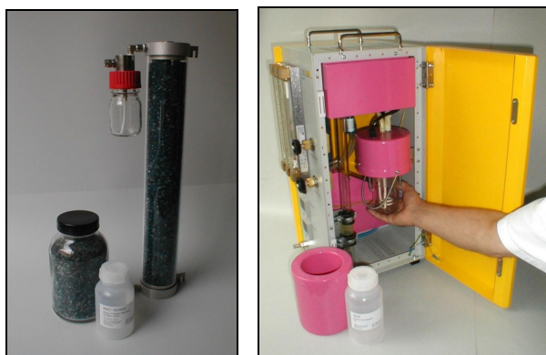
Left: Dismounted Nuclei Source (Atomizer and Diffusion Dryer) for Replacing Dessicant (Silicagel) through the Inlet on the Top Right: Removing Saturator Vessel for Refilling with Particle Material
