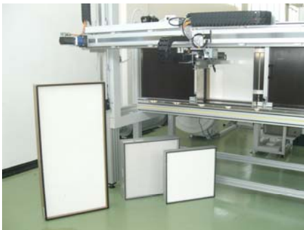
Filter holder cabinet with scanning traverse
