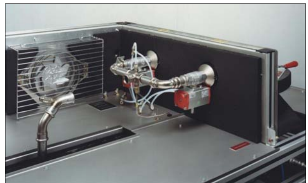
Test chamber (opened) with upstream and downstream test piece connectors, being adjustable for different test object sizes. Integrated in the rear plate the heater blower combination.
