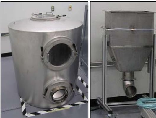
Stabilization vessel and universal panel filter holder
