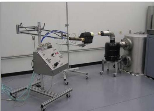
Water injection system and water separator
