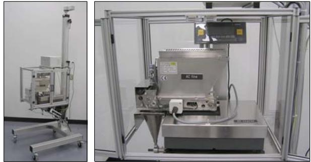
Dust feeder SAG 420 with scale and housing
