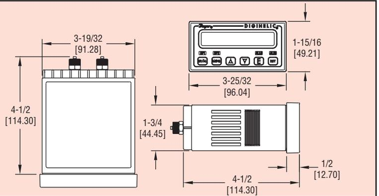
The Series DH Digihelic® Differential Pressure Controller is a 3-in-1 instrument possessing a digital display gage, control relay switches, and a transmitter with current output. Combining these three features allows the reduction of several instruments with one product, saving inventory, installation time and money. The Digihelic® Controller is the ideal instrument for pressure, velocity and flow applications, achieving a 0.5% full scale accuracy on ranges from 5 to 100 in. w.c.
